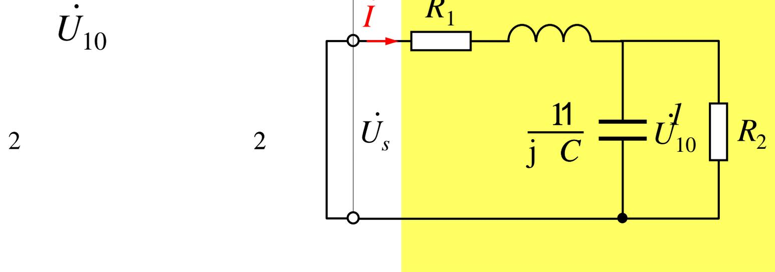
$$\dot{U}_{10} = Z_{10} \dot{I} = 303.45 \cdot 0.6 \angle 72.33^\circ = 182.07 \angle -20.03^\circ \text{ V}$$
