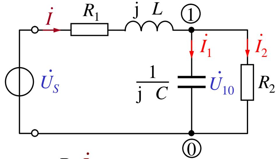
$$\dot{U}_{10} \xrightarrow{\text{VCR}} \begin{Bmatrix} \dot{I}_1 \\ \dot{I}_2 \end{Bmatrix} \xrightarrow{\text{KCL}} \dot{i} \xrightarrow{\text{VCR}} \begin{Bmatrix} R_1 \dot{I} \\ j L \dot{I} \end{Bmatrix} \xrightarrow{\dot{U}_{10} \text{ KVL}} \dot{U}_s$$
