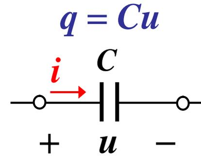
$$i = \frac{dq}{dt} \quad q(t) = \int_{t_0}^t i(\xi) d\xi = \int_{t_0}^{t_0} i(\xi) d\xi + \int_{t_0}^t i(\xi) d\xi$$
