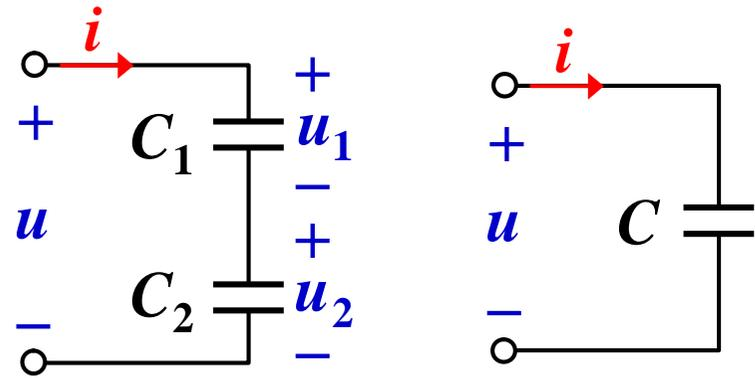
$$C = \frac{C_1 C_2}{C_1 + C_2}$$
